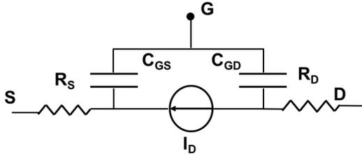
Fig. 8. The CNT-TFT compact model.
