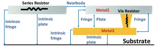
Fig. 15. Different types of parasitic capacitors and resistors.
