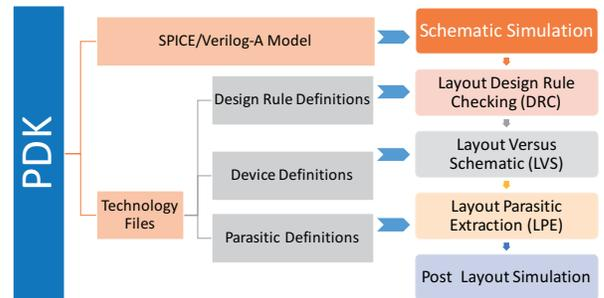
Fig. 7. Process Design Kit (PDK) provides necessary information for the circuit design.
