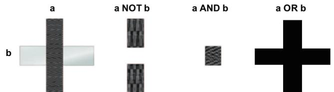
Fig. 12. Common boolean operations of layer a and b. Boolean operations: NOT, AND and OR are demonstrated.
