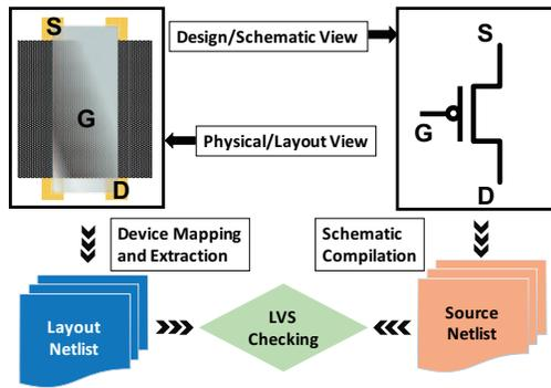
Fig. 14. LVS principles and procedures.
