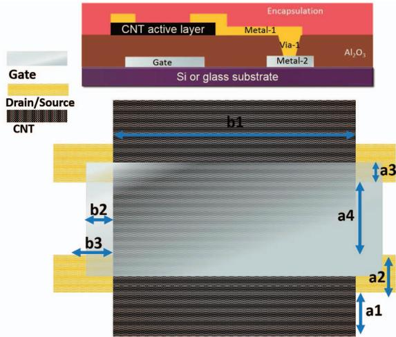
Fig. 2. (Top) Side view of a carbon nanotube transistor (CNT-TFT). (Bottom) Top view of a CNT-TFT including physical dimensions for DRC.
