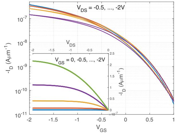
Fig. 3. Drain current versus gate voltages for a CNT-TFT.
