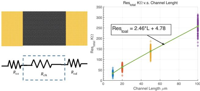
Fig. 10. Flexible resistor analysis based on  $\approx 500$  fabricated devices with  $L = 10, 20, 50, 100 \mu m$  and  $W = 40 \mu m$ .
