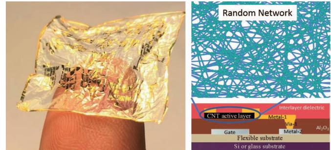
Fig. 1. (Left) A CNT-TFT logic circuit on a 1- $\mu\text{m}$  thick plastic foil. (Right) Side view of a CNT-TFT [1].
