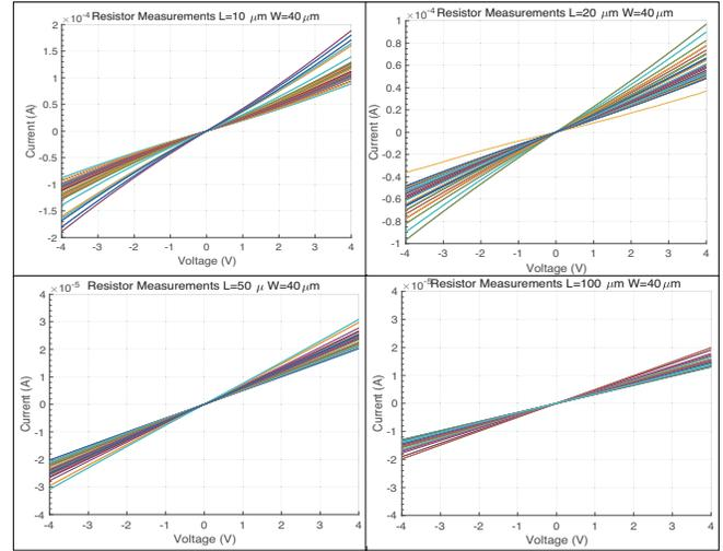
Fig. 6. Measured I-V characteristics of flexible CNT resistor array. The width is 40- $\mu\text{m}$  and the length varies from 10- $\mu\text{m}$  to 100- $\mu\text{m}$ .
