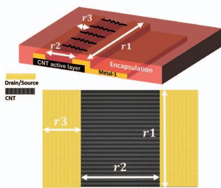
Fig. 5. Device dimension of a CNT resistor.  $r_1$  represents the device width  $W$  and  $r_2$  represent the device length  $L$ .  $r_3$  is the metal enclosure distance.
