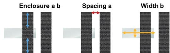
Fig. 13. Common checking statements: enclosure, spacing and width.
