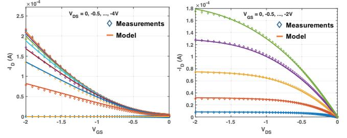
Fig. 9. Model validation for  $I - V$  curves.
