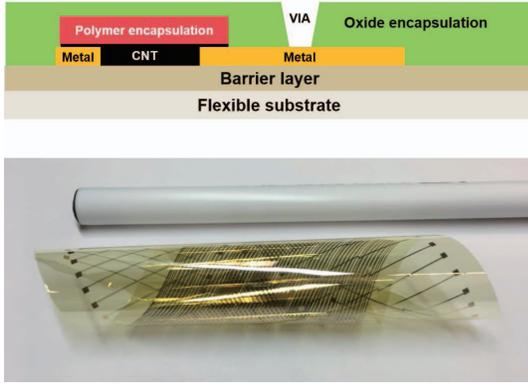
Fig. 4. (Top) Side view of a CNT resistor. (Bottom) Device photo of the CNT resistor array on a 10- $\mu\text{m}$  thick polyamide foil.
